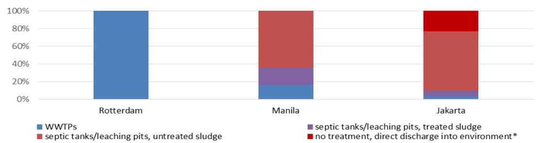
**Figure 2** Sewage management overview for Rotterdam, Manila and Jakarta. (\*Direct discharge includes pit latrines/toilets that discharge directly into ditches and drains and also the toilet waste from the population that doesn't have any facility).
